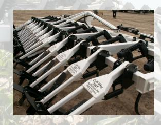
Free floating design for better ground contact and uniform pocket depth
